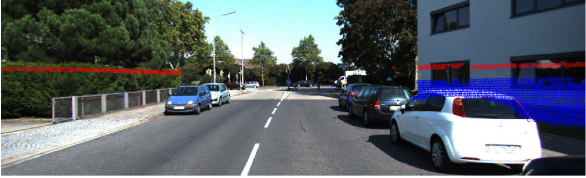
(a) Here, foreground points (in blue) are determined to be similar to known background points (in red).
