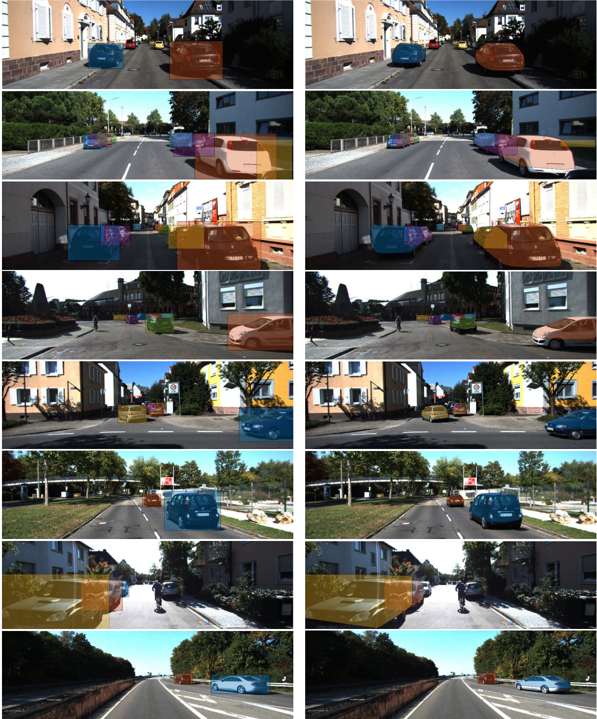
Figure 4.6: Resulting refinement of neural network bounding box proposals. Left column is neural network proposals. Right column is heuristic refinements.
