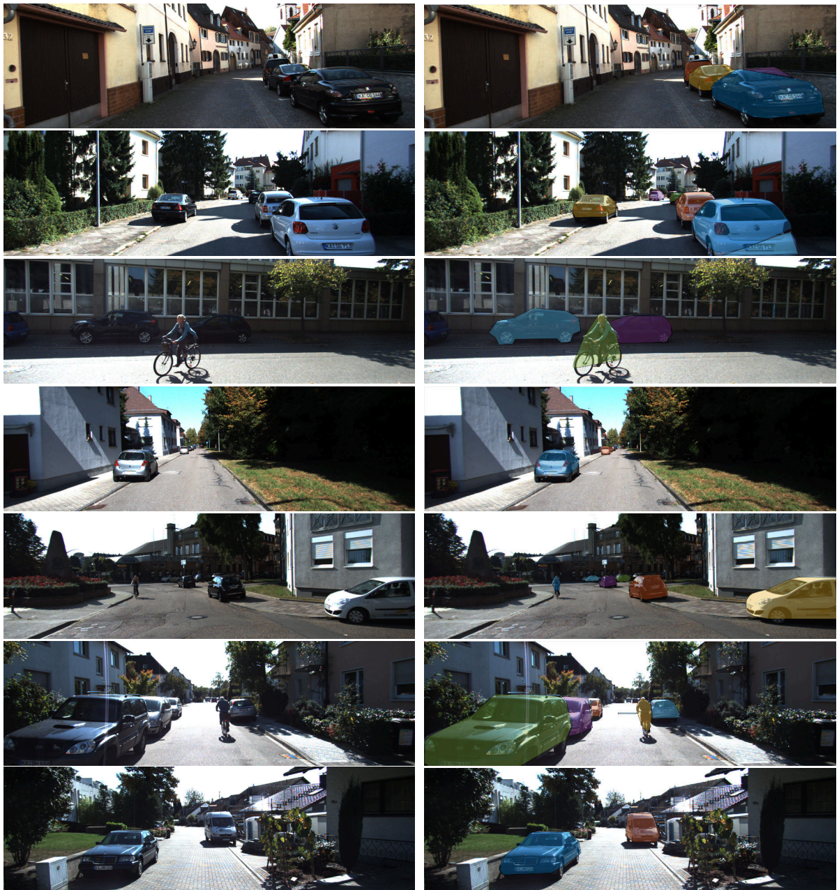
Figure 4.5: Resulting segmentations. Left column is original image. Right column is original image with segmentations over-layed.
