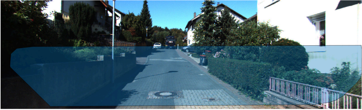
Figure 5.4: Height threshold failure on an incline. Here, the road is incorrectly added to persistent foreground clusters.
